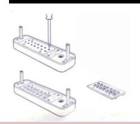
Failure to follow the instructions could result in damage to your lock so please read carefully. Hold the outside body in the horizontal position. Remove the 4 red screws. Carefully remove the plate, as there are many springs attached to.
