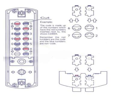
Using the tumblers provided, the code can be changed from a 3 digit to a 7 digit number, always prefixed by C to clear. To increase the numbers in the combination, remove the **blue** and add the red tumblers. To decrease the numbers in the combination, remove the red tumblers and add the blue. (If you insert a tumbler in the wrong position, press the C button and lift the tumbler out.)
